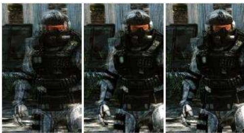
Figure 4: Left: Using a naive resolve results in visible ghosting. Middle: Reprojection mitigates these artifacts but does not completely remove them. Right: The addition of velocity weighting allows to completely remove ghosting.
